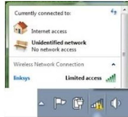
**FIX 1:** Make sure your laptop's wireless card is turned on. There is a button on the top row that toggles Wi-Fi off and on (varies by model). If there is an orange light on that button, the Wi-Fi card is turned off. Press that button and it should turn white or turn off. On keyboards where this symbol is in a box (below), you may need to press the **Fn** button on the keyboard and hold it down while pressing the Wi-Fi button.
